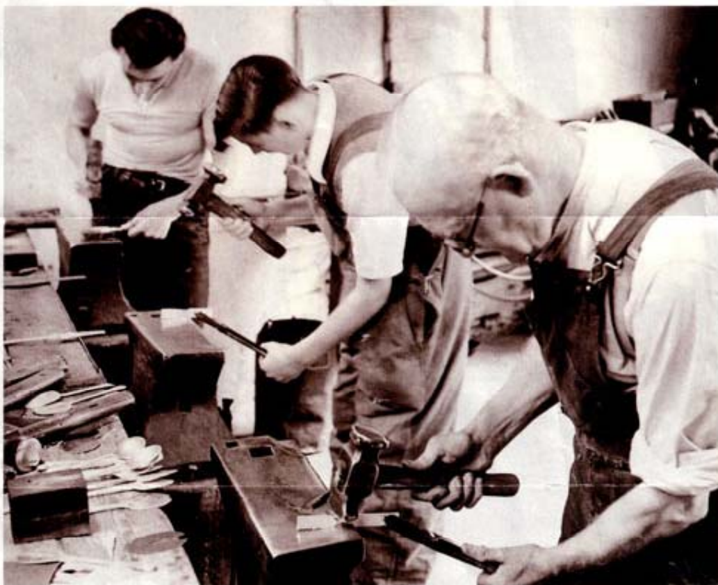
THE WAY IT WAS—AND STILL IS Hand-hammering by craftsmen at the Fletcher workshop in Sheffield, England (ca. 1970), condenses the silver, making it heavier, more durable, and perfectly balanced.
